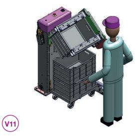
Left side loading, lengthwise, tilting to the front
