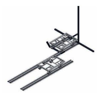
Slide mechanism - change of rail
