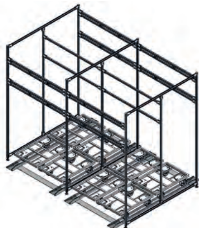
Top structure with conveyor belt on shelf
